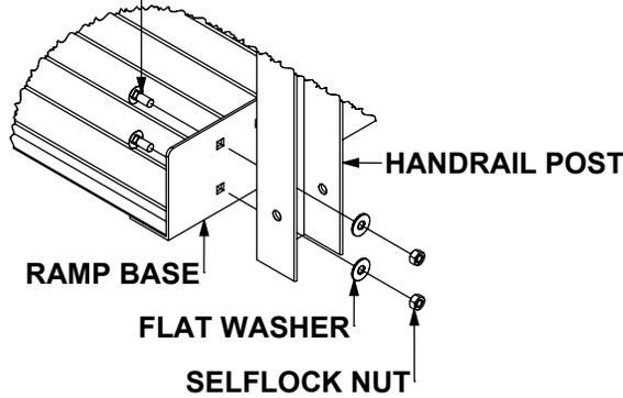
**STEP#2:** Attach handrails to ramp base by placing carriage bolts through the ramp frame and the handrail post and fasten with flat washers and selflock nuts. If handrail post is at a splice location place carriage bolts through the ramp frame, the ramp splice, and the handrail post. Before attaching next section of handrail place handrail splice inside of handrail tube to splice top handrail tube together.
