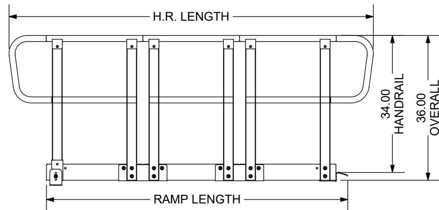
**STEP#1:** Splice ramp base sections together using the ramp splice by running a carriage bolt through the square holes in the frame rail of the ramp base and round holes of the ramp splice, fasten with flat washers and selflock nuts.
