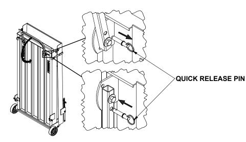
**STEP#1**: Stand ramp upright and remove quick release pins from handle. Fold handle down and replace quick release pins to lock handle in place.
