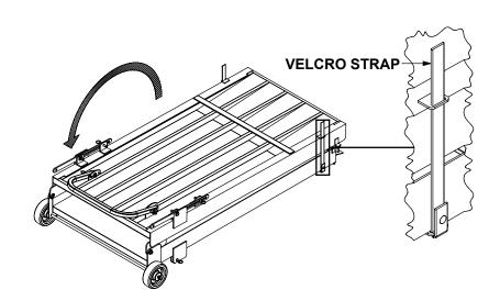
STEP#2: Lay ramp flat with the hook side down and undo Velcro straps, and unfold ramp. DO NOT UNDO VELCRO BEFORE LAYING THE RAMP FLAT DOING SO COULD RESULT IN INJURY.
