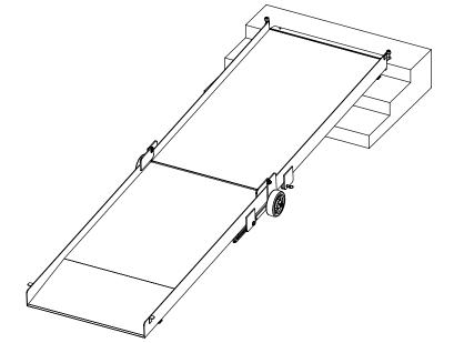
**STEP#4:** Move ramp into position for use making sure the hook is positioned correctly on step. Use pins provided to anchor ramp to step. Holes for pins will need to be drilled. **DO NOT USE RAMP UNLESS IT HAS BEEN ANCHORED DOWN.**
