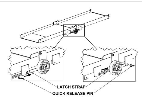
**STEP#3:** Remove quick release pins from bottom assembly on each side of the ramp, and slide latch straps forward and align holes in latch strap with top assembly and replace quick release pins.
